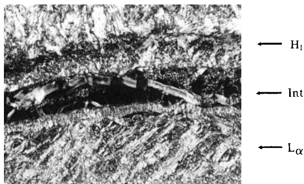
Figure 5. Penetration scan for HDOB (70°C). (Top -H 1 ; middle-intermediate; lower-L α . Sample size c. 0.4 × 0.5 mm).
